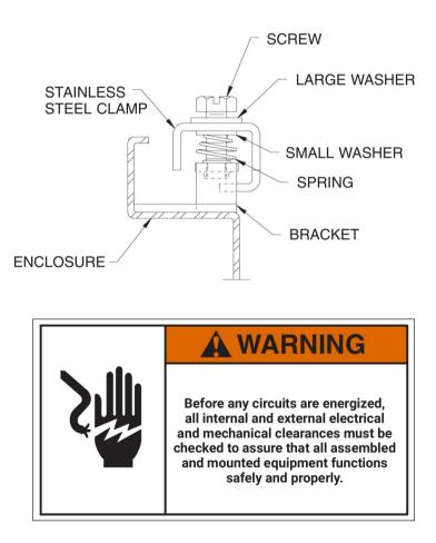
This accessory maintains UL/CSA Type 12,4,4X when installed per these instructions. This accessory is covered by UL file E61997 and CSA file LR42186.
